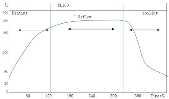
Heating: $25^{\sim}150^{\circ}\text{C}$ ,  $2-3^{\circ}\text{C/sec}$ Reflow:> $150^{\circ}\text{C}$ ,  $180-240^{\circ}\text{sec}$
